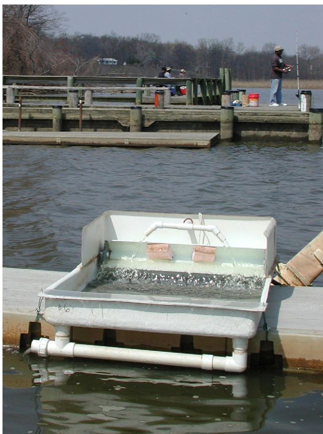
Fig. 1. Photograph of algal turf scrubber unit on a dock at the Patuxent River Park on the Patuxent River.
