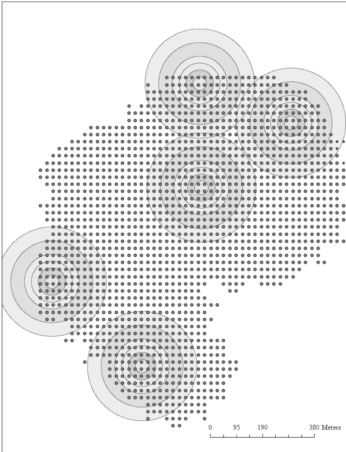
Figure 4. Location of the water quality stations and their buffers of different diameters. Grey dots represent the locations of 2500 points that predict vegetation density throughout the marsh through kriging. The buffers allow to test whether vegetation density and water quality are related at different spatial scales.
