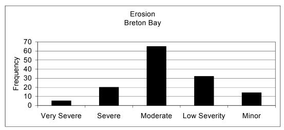
Figure 5b Histograph showing the frequency of severity ratings given to erosion sites during Breton Bay SCA survey.
