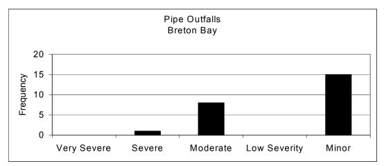
Figure 9b Histograph showing the frequency of severity ratings given to pipe outfall sites during Breton Bay SCA survey.
