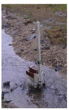
Figure 3-2. Siphon sampler
