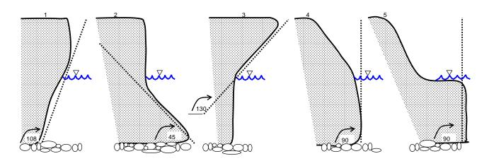
Figure 7. Bank angle scenarios (perspective: cross-section view)(Rosgen 2003).
