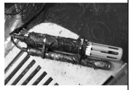
YSI sonde with copper anti-fouling sensors and sonde guard deployed for more than 1 month during the summer in Puget Sound. Photo courtesy of Stephanie Hess, King County.
