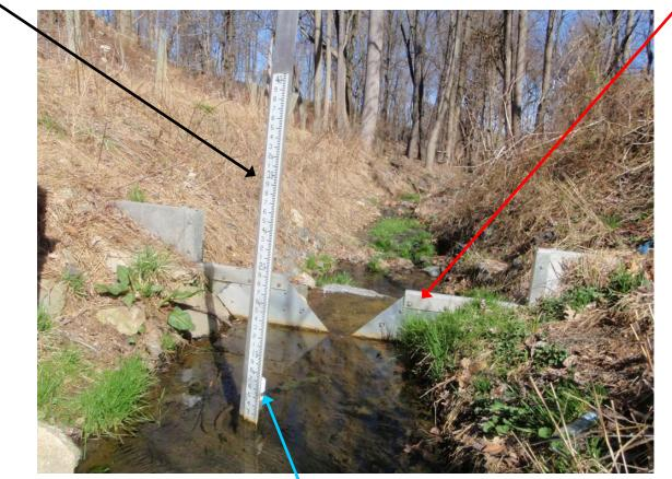
pressure transducer (inside pvc pipe)
