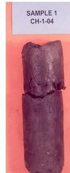
Core samples of grout that cured inside the mine.
