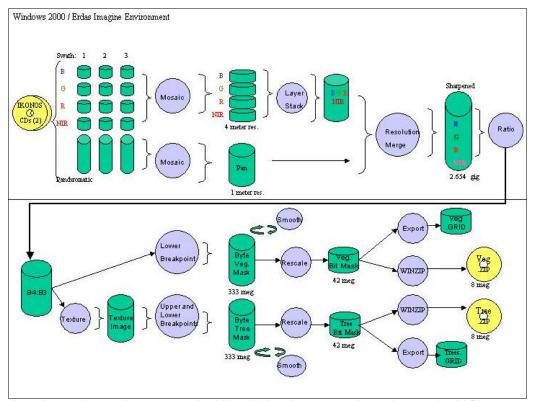
Figure 3. Procedure used to convert IKONOS bundled product to vegetation and tree mask grid files. Braces and arrows both represent direction of work flow. Circles represent ERDAS Imagine application programs or models.
