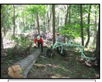
Operator hooking cable to pull log under arch before skidding.
