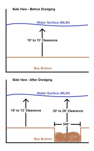
Figure 1b. A stylized cross section of the proposed dredge cuts to be made at Man-O-War shoal. Actual cut sides and bottoms are not at precise right angles.
