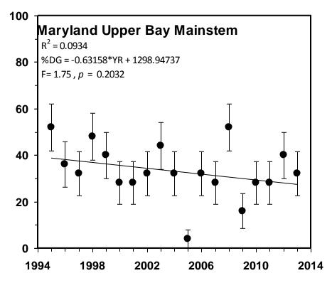
Figure 10. Proportion of the Maryland upper bay mainstem strata (+/- 1 standard error) with degraded (total area failing restoration goals) benthic community condition. Trends of temporal changes tested by ANOVA. From Llanso et al. 2014
