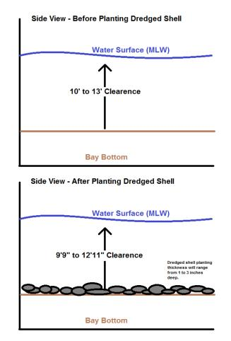
Figure 14: A generalized cross section of planting dredged shell.
