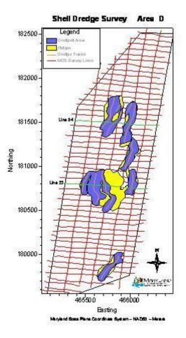
Figure 8. Sonar track lines from the 2006 survey conducted by Maryland Geology Services.
