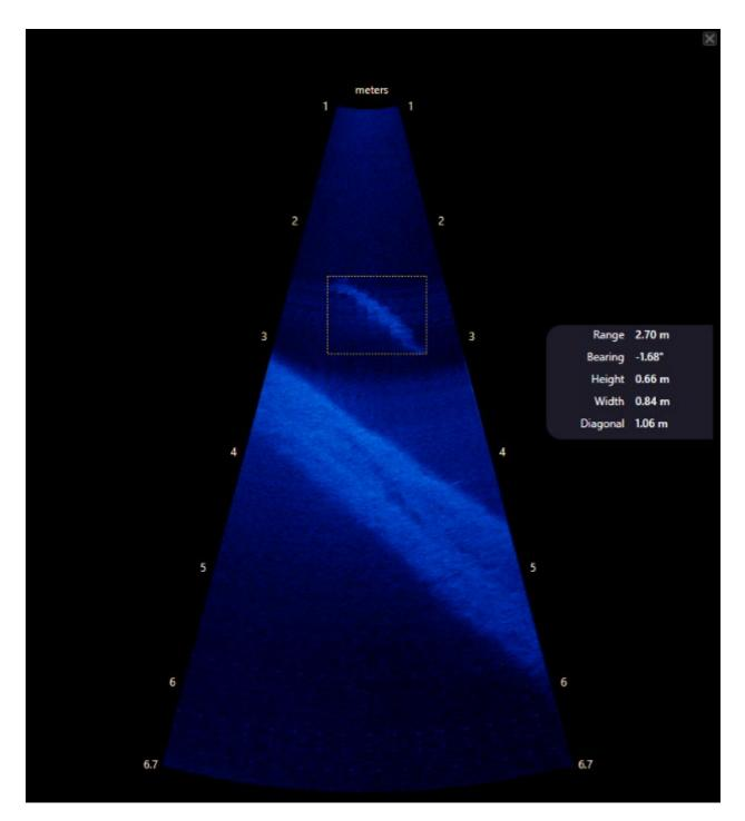
Figure 4.2. Detection of a possible sturgeon as seen in ARIS data recorded on 26 September 2019 near the Route 313 Bridge, Brookview MD. The fish is indicated by the yellow bounding box and is approximately 1.06 m long, as indicated by the length of the diagonal of the bounding box. It can be seen moving through the water column approximately 3m from the camera lens.
