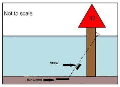
**Figure 4**. Maryland Department of Natural Resources methodology for attaching receivers to United States Coast Guard fixed piling aids to navigation.
