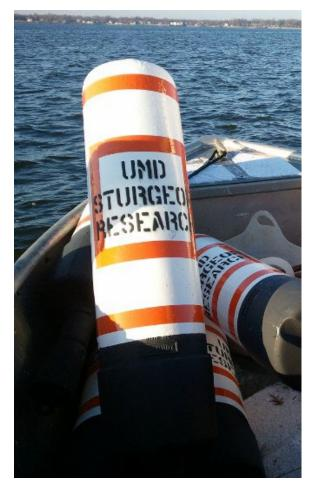
**Figure 6**. Maryland Department of Natural Resources Jim-Buoy<sup>®</sup>. These buoys are used to place acoustic receivers in specific locations when no USCG fixed pilings or private piers could be located.
