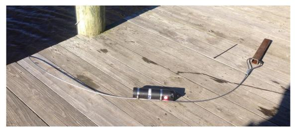
**Figure 5**. Maryland Department of Natural Resources methodology for attaching acoustic receivers to stainless steel cable on the Nanticoke River and Marshyhope Creek.
