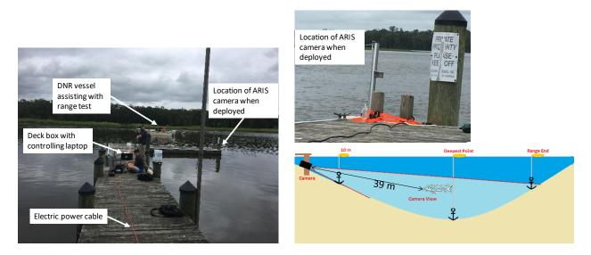
Figure 3.1. Deployment (26 August 2019) of ARIS camera at Henson Scout Reservation near the mouth of the Marshyhope Creek. ARIS camera was deployed on a floating pier at the end of a long fixed pier, held in place by a specially fabricated pipe-bracket assembly and ratchet straps. Also shown is conceptual figure of camera angle adjustments made to try to maximize river bed coverage.
