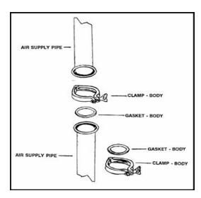
Figure 3 – Sanitary Pipe Fitting
