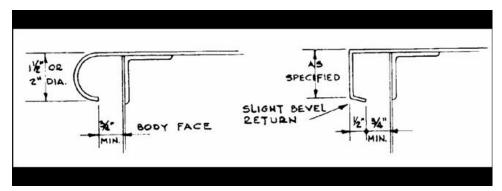
Figure 19 – Exposed edges and nosings on horizontal surfaces
