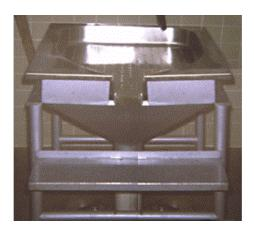
Figure 10 – Photo front view of a skimmer
