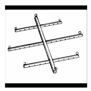
Figure 9 – Air manifold located inside tank
