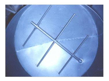
Figure 8 – Air manifold installed inside the blower tank
