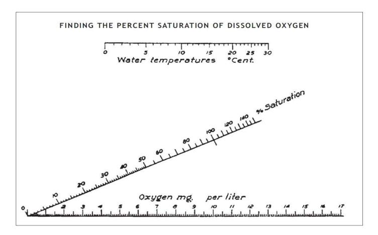
To read this chart, use a straight edge. Place the straight edge on the mg/L of oxygen you have determined for your site, then place the other end of the straight edge on the water temperature you have measured. The point where the straight line passes through the line labeled "% Saturation" is your percent saturation.
