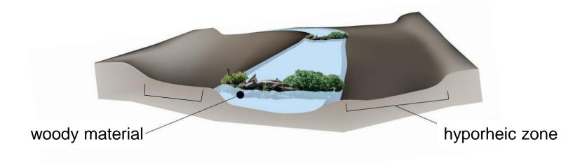
4. The channel plan form design, with characteristic large meanders, small channel widths and depths, and developing multiple flow pathways, results in increased groundwater and surface water flow retention, as well as increased exchange between stream channels and adjacent hyporheic zones.
