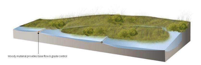
To provide additional denitrification potential and other habitat benefits, stumps and woody material placed in restored floodplain areas increases roughness during flooding and promotes trapping of additional organic debris during high flows.
