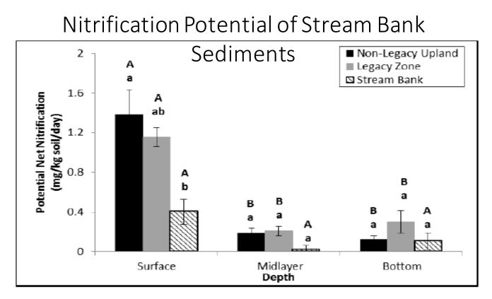
Figure 4-2: Potential net nitrification rates expressed as averages across landscape positions and depths. Vertical bars denote one standard error of the mean. For a given depth, bars with different lowercase letters represent statistically significant (p < 0.05) differences between land positions. For a given land position, bars with different uppercase letters represent statistically significant (p < 0.05) differences tatistically significant (p < 0.05) differences with depth.
