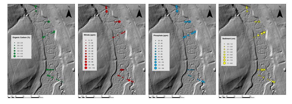
Distribution of C, NO<sub>3</sub>, PO<sub>4</sub> & Sediment on the Restored Floodplain
