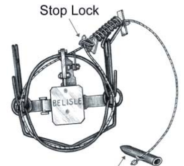
Coil-Spring Activated Cable Device
