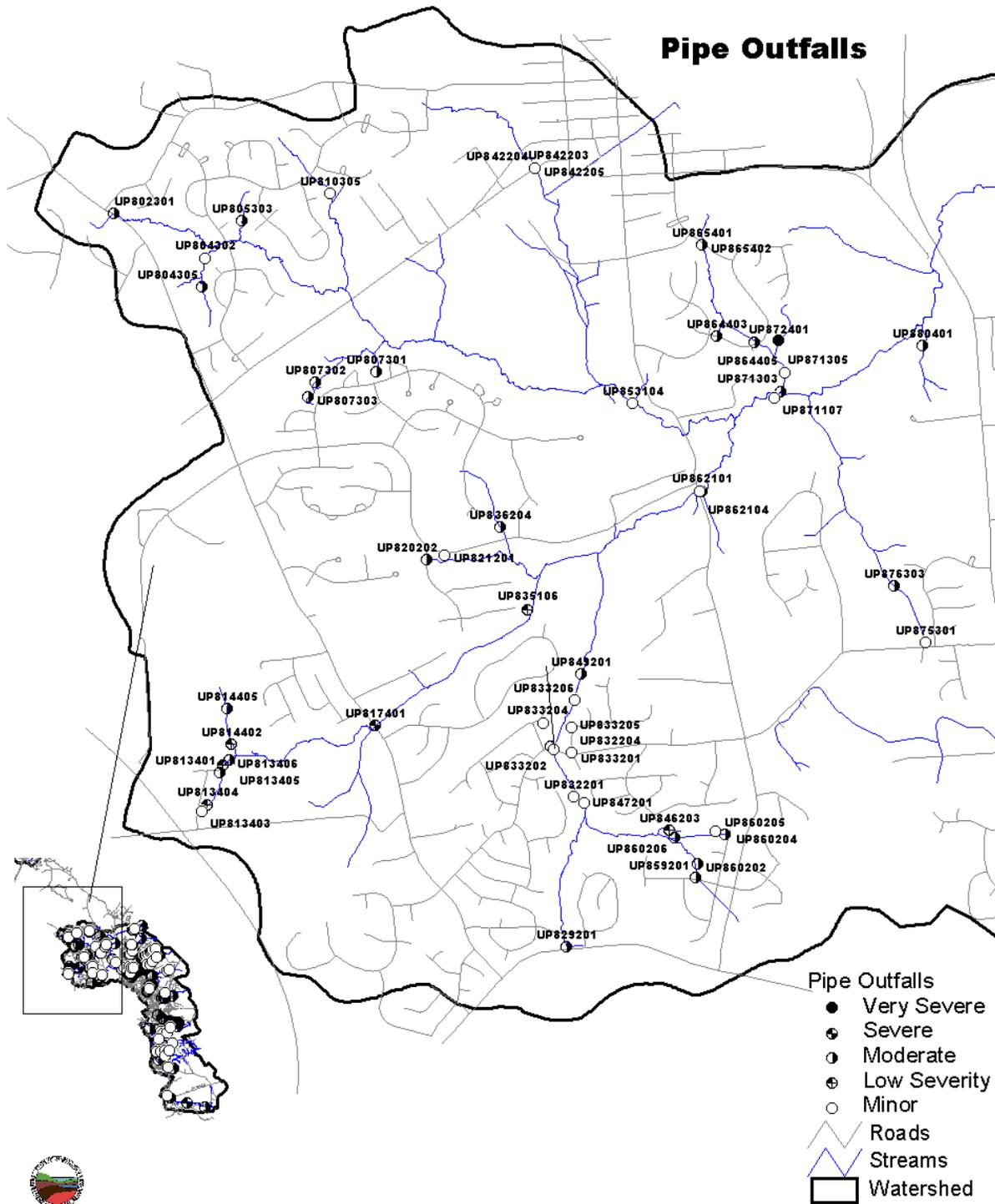
Figure 5c: Map showing the Pipe Outfalls locations in one section of the Prince George's Upper Patuxent Watershed
