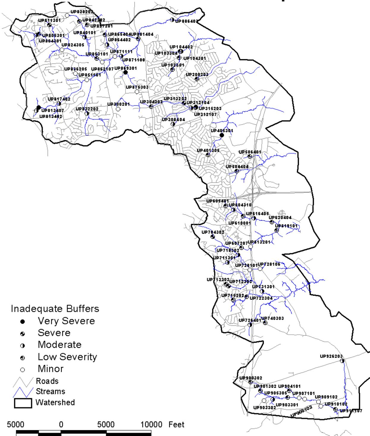
Figure 8: Map showing the Inadequate Buffer locations in the Prince George's Upper Patuxent Watershed
