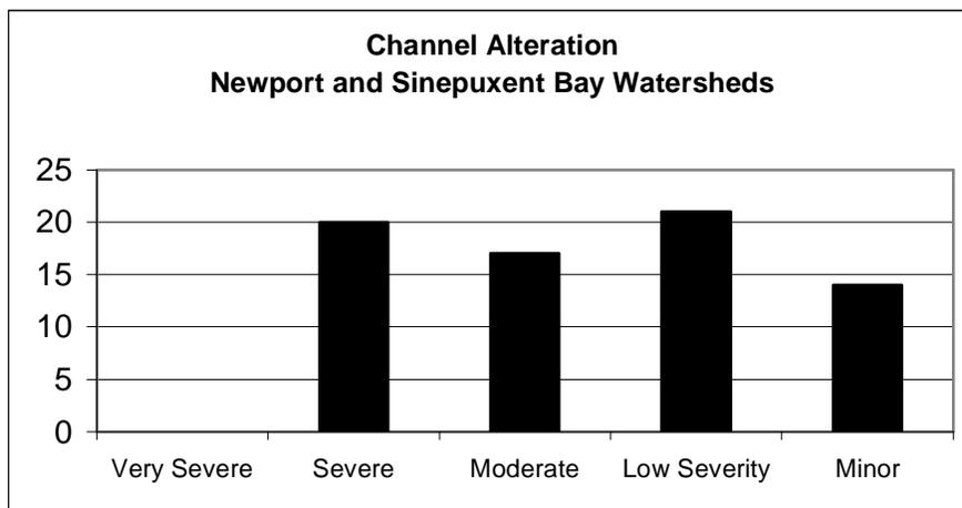
**Figure 4b. Histogram showing the frequency of severity ratings given to channel alteration sites during the Newport and Sinepuxent Bays' SCA survey.**
