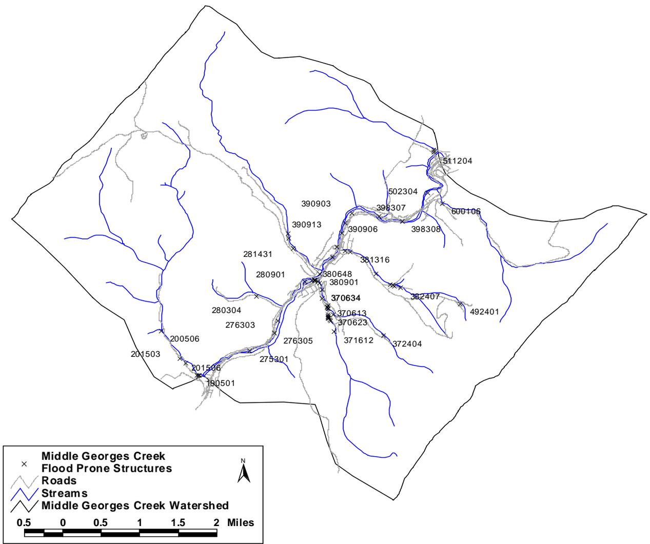
**Figure 9b: Middle Georges Creek Flood Prone Structures.**
