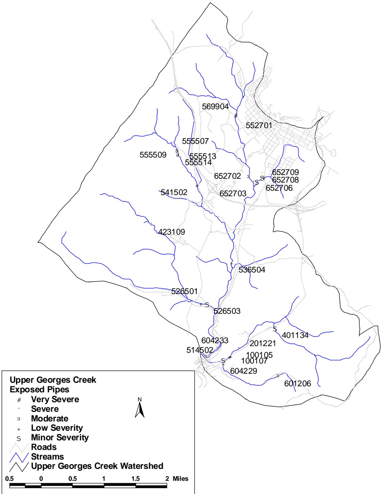
Figure 10b: Upper Georges Creek Exposed Pipes.
