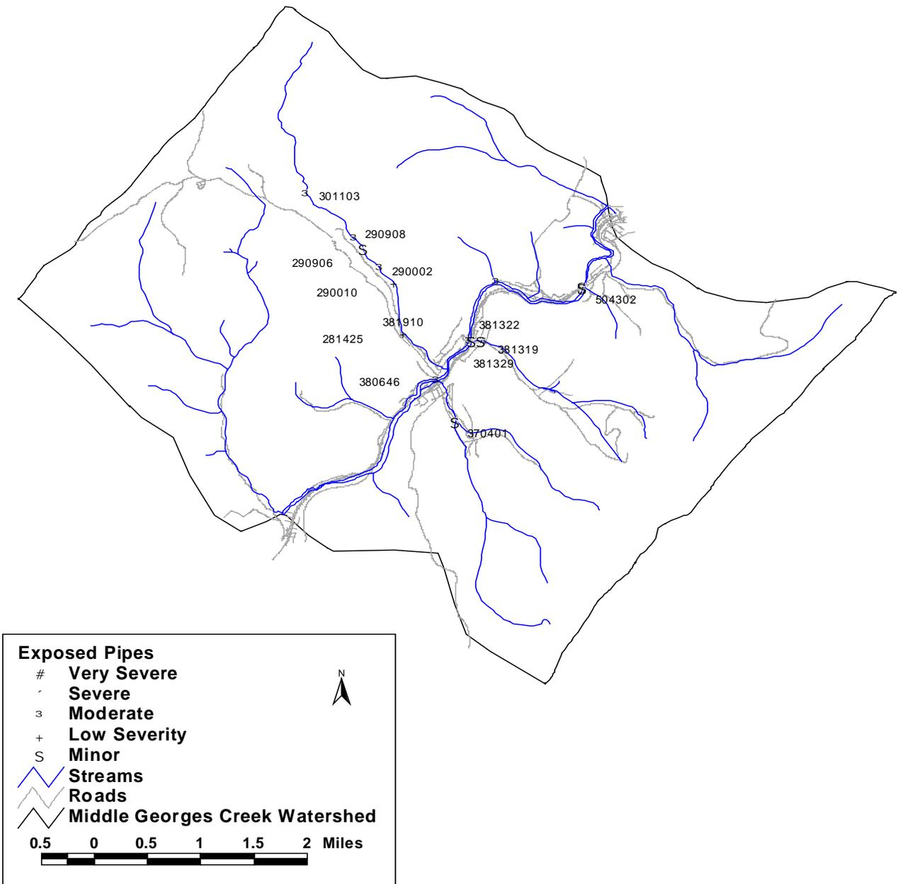
**Figure 10c: Middle Georges Creek Exposed Pipes.**
