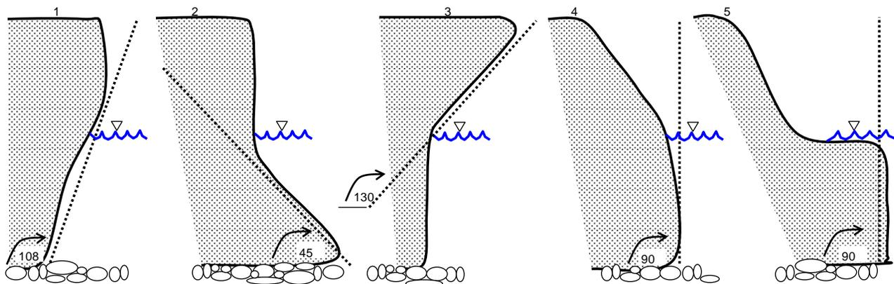
Figure 7. Bank angle scenarios (perspective: cross-section view)(Rosgen 2003).
