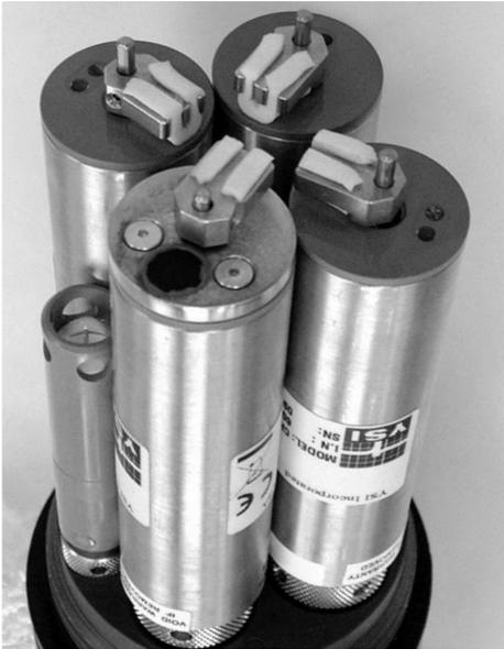
YSI sonde equipped with copper-alloy anti-fouling kit was deployed in the Arabian Gulf for 3 months. Copper has chemical properties that deter biofouling from adhering and growing on the sonde's surfaces.
