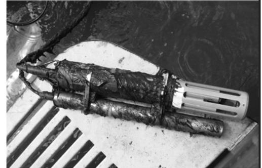
YSI sonde with copper anti-fouling sensors and sonde guard deployed for more than 1 month during the summer in Puget Sound. Photo courtesy of Stephanie Hess, King County.
