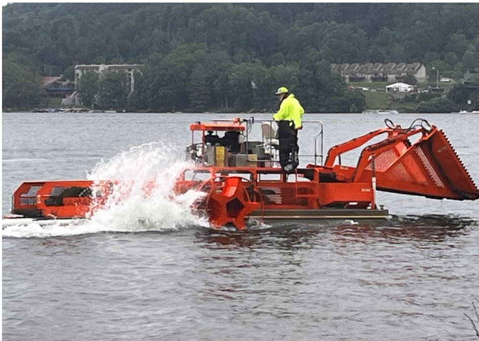
Figure 1: Model H5-200 aquatic vegetation harvester on Deep Creek Lake.
