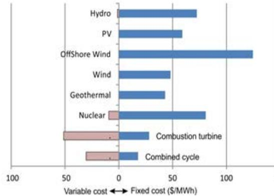
Figure 1 Fixed vs variable generation cost
