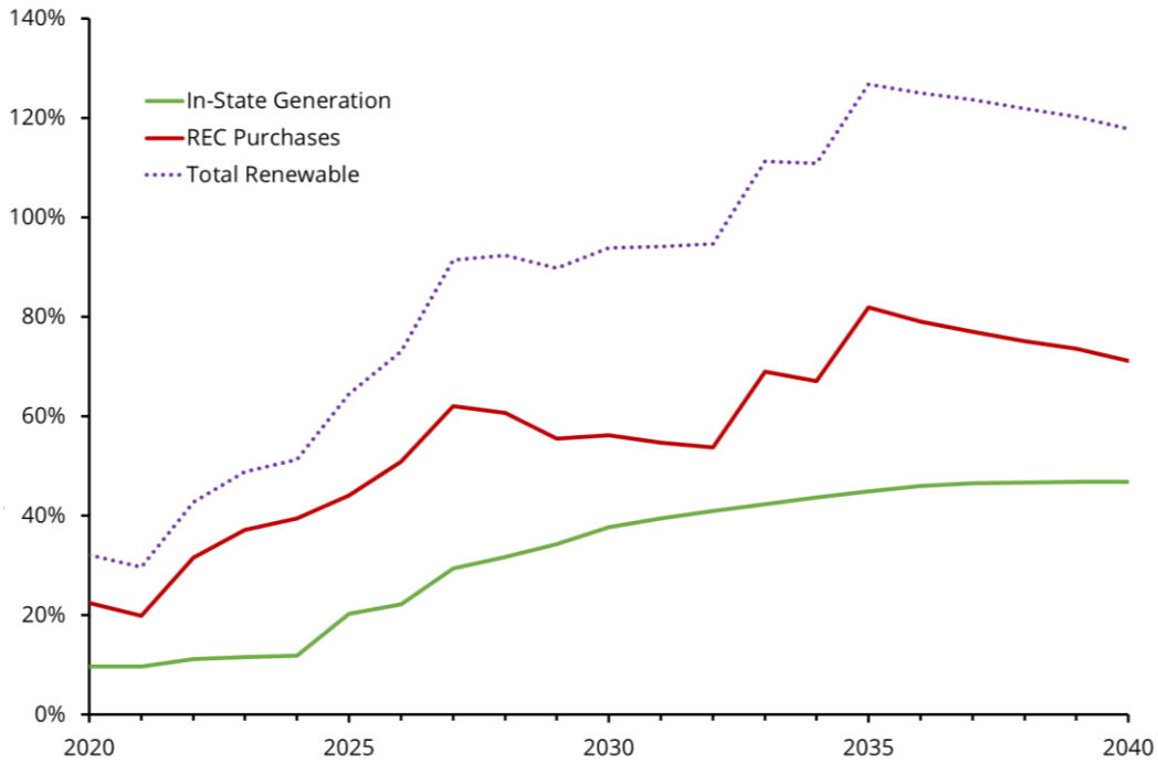
Figure 35. Proportion of Maryland Demand Met by REC Purchases Versus In-state Generation, 100% RPS-1 Scenario
