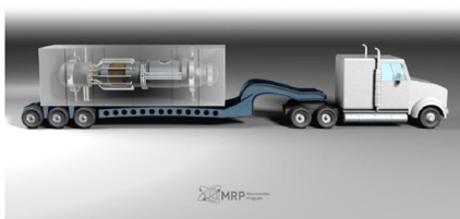
Microreactors can be easily transported by truck.
