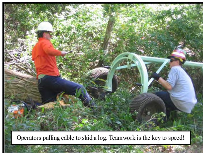
Operators pulling cable to skid a log. Teamwork is the key to speed!
