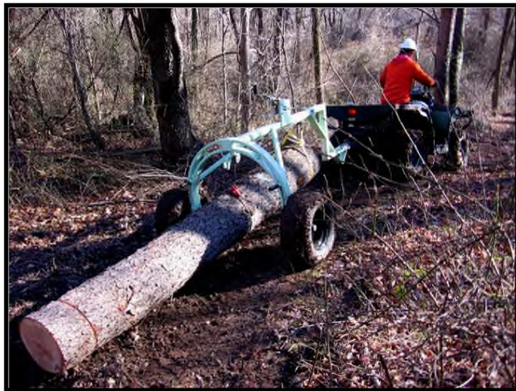
Operator at work with ATV & skidding arch - notice minimal disturbance.
