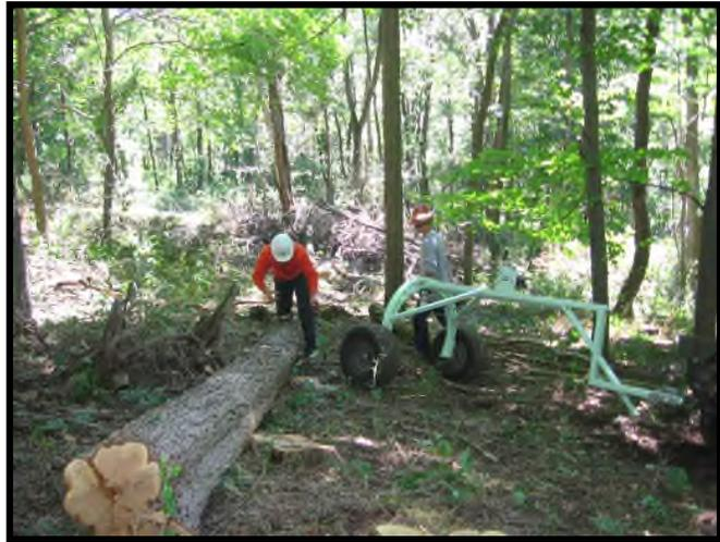
Operator hooking cable to pull log under arch before skidding.
