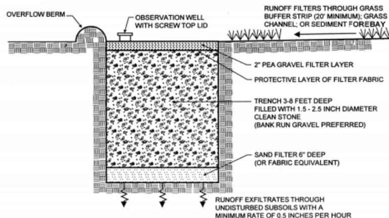
Figure 1. Profile of an infiltration system. Source: Maryland Stormwater Design Manual, MDE
