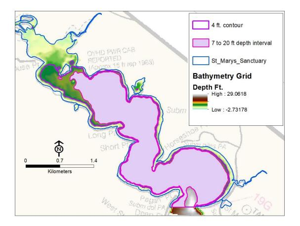
Depth data for the St. Marys Sanctuary. The U.S. Army Corps of Engineers Master Plan absolute criteria for maximum depth is 20 feet MLLW.
