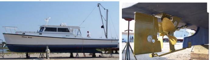
Drydocked R/V Miss Kay for scheduled maintenance and repairs. Modified vessel skeg for reduction of propeller cavitation, waxed vessel hull, cleaned bottom and painted same with anti-fouling paint, installed new safety bow railing pulpit, recoated all sub-surface metal works with "Prop-Speed" anti-fouling epoxy application, installed new fuel tank thru-hull vents, propeller reconditioned, pitch reset and new propeller drive shaft installed.
