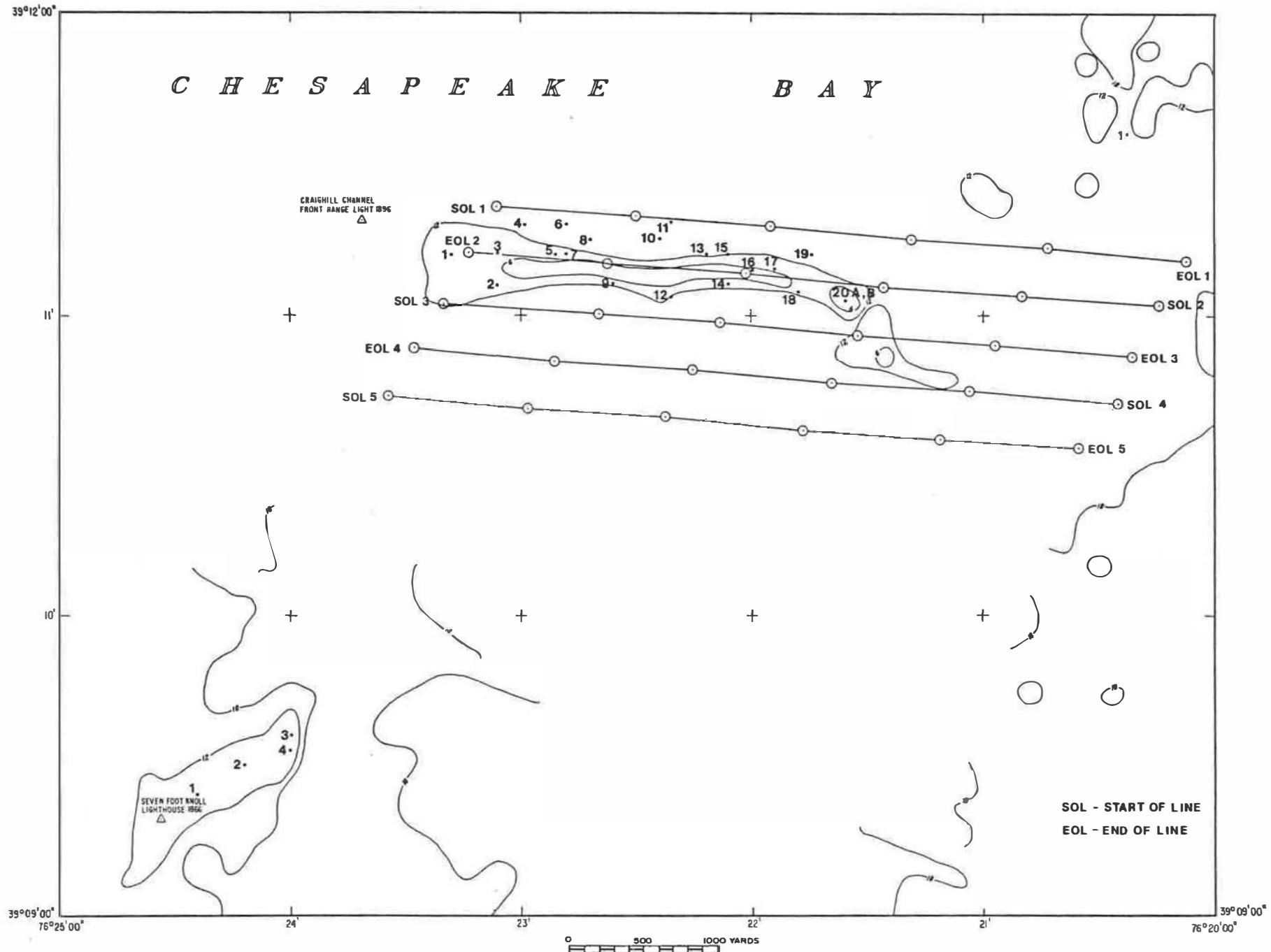
**FIGURE 3.** CHART SHOWING TRACK LINES FOR SEISMIC SUBBOTTOM RECONNAISSANCE IN VICINITY OF SIXFOOT KNOLL.
