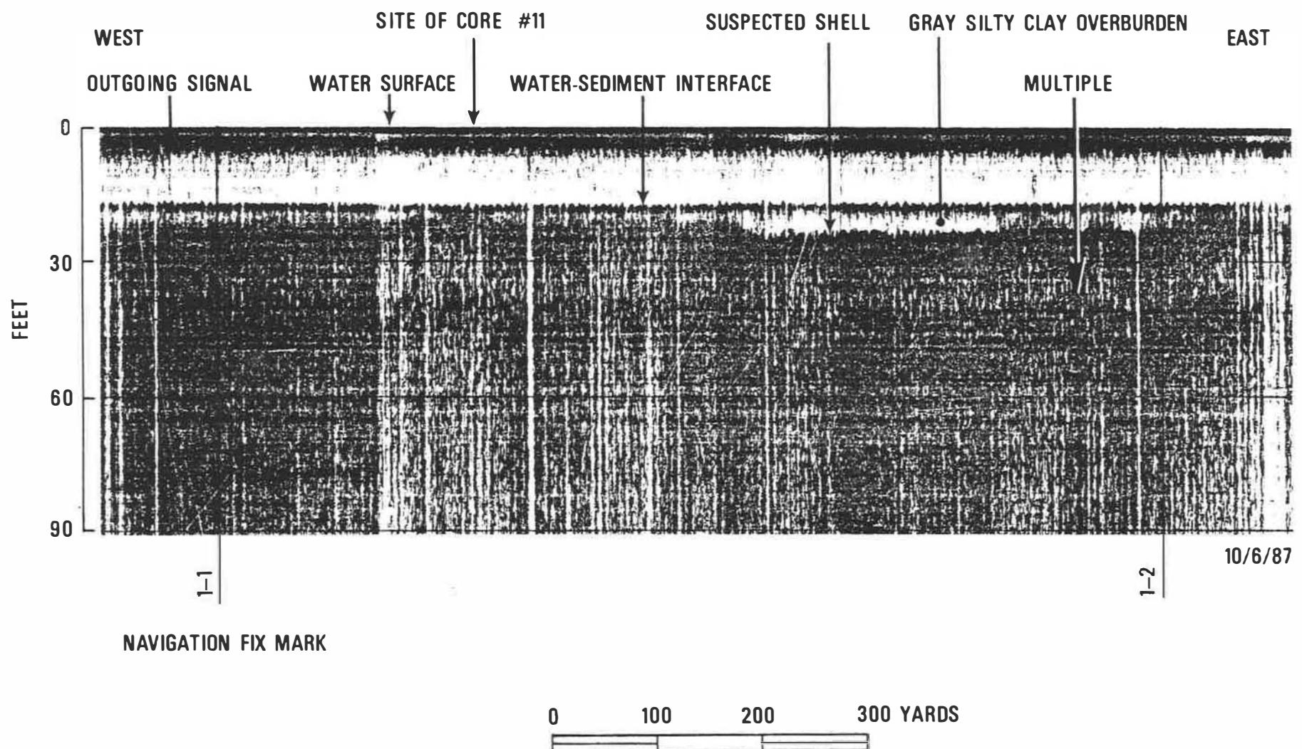
**FIGURE 6.** SECTION FROM SEISMIC RECORD ALONG TRACK LINE 2 AT MAN O'WAR SHOAL (BETWEEN FIX MARK 5 AND END OF LINE) WITH CORE #3 LOCATION INDICATED.
