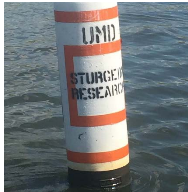
Figure 5. A Maryland DNR Jim-Buoy deployed with the acoustic receiver attached. The Jim-Buoy was anchored with two 22 kg cement anchors by a length of galvanized chain approximately 3 m longer than the depth at high tide. The receiver was attached to an eye bolt on the bottom of the Jim-Buoy with the primary acoustic receiver attachment method (Figure 1).
