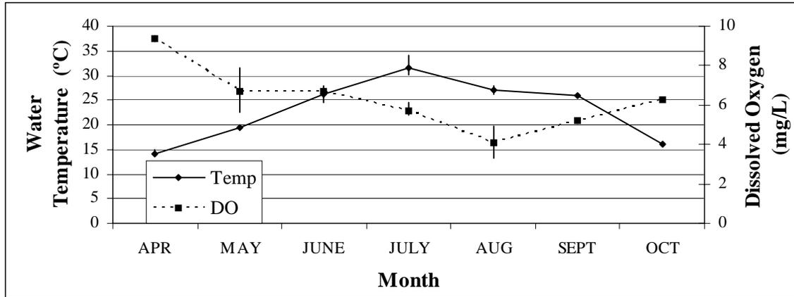
Figure 166. 2005 Coastal Bays Fisheries Investigations Trawl Survey mean water temperature (°C) and dissolved oxygen (mg/L) in Assawoman Bay. Error bars represent the range of values collected.
