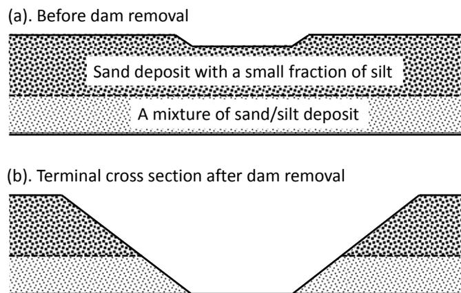
**Figure 8.** Sketch showing idealized sediment deposit and erosion following dam removal in the DREAM-1 model, in which sand and silt are combined as layers of sand/silt mixture.
