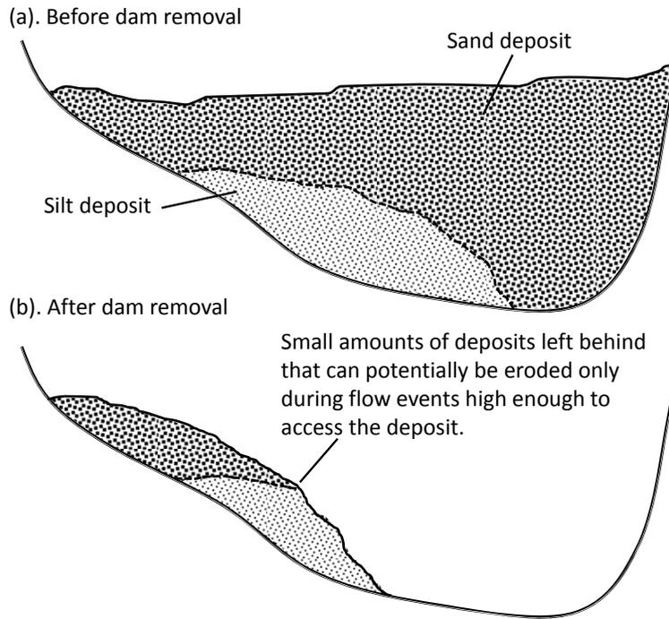
**Figure 7.** Sketch of the sediment deposit in Bloede Reservoir before and after dam removal, showing that a small amount of sediment deposit may be left behind in the former reservoir area following dam removal, with potential erosion occurring only during high flow events when the deposit is accessed by the flow.
