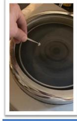
**STEP 3.** PLACE THE UNPOLISHED END INTO CLAY AND PLACE THE POLISHED END BENEATH THE LENSE OF A DISSECTING MICROSCOPE (OR A STEREOSCOPE).
