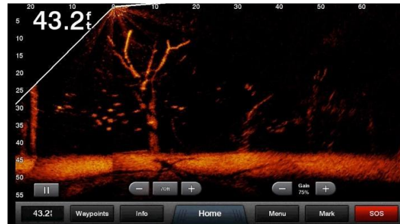
A screenshot of the display screen from live-imaging sonar showing a school of fish on submerged timber.
