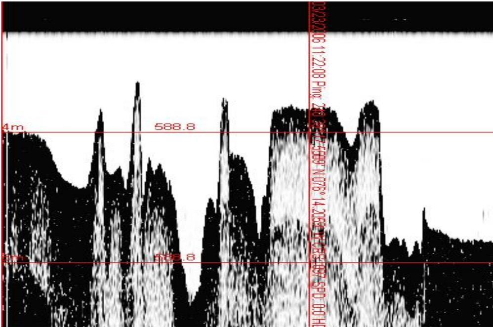
Figure 9. Vertical profile along a survey track line, shown in green in Figure 8, in Area D. The water surface is the thick black line at the top of the image. The horizontal scale is tightly compressed compared to the vertical scale. Cuts are generally 10' to 15' deep and hundreds of feet wide. This image shows cuts and also undredged ridges and peaks are left between cuts.
