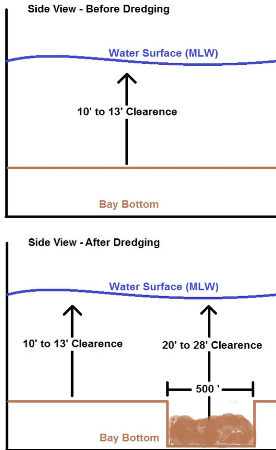
Figure 1b. A stylized cross section of the proposed dredge cuts to be made at Man-O-War shoal. Actual cut sides and bottoms are not at precise right angles.
