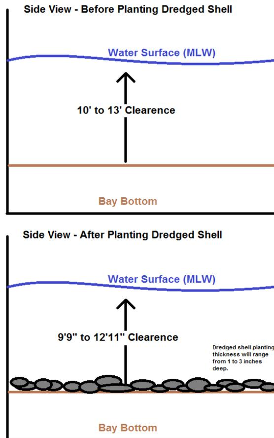
Figure 14: A generalized cross section of planting dredged shell.
