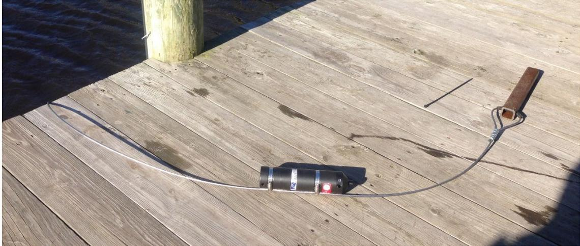
**Figure 5.** *Maryland Department of Natural Resources methodology for attaching acoustic receivers to stainless steel cable on the Nanticoke River and Marshyhope Creek.*
