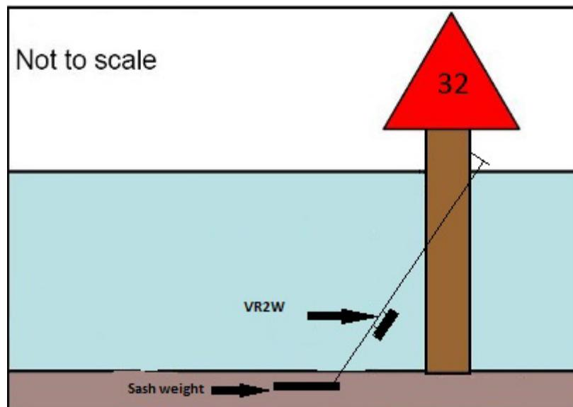
**Figure 4.** *Maryland Department of Natural Resources methodology for attaching receivers to United States Coast Guard fixed piling aids to navigation.*
