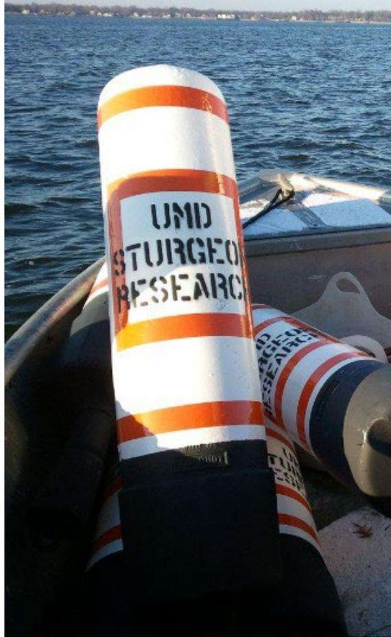
**Figure 6.** *Maryland Department of Natural Resources Jim-Buoy®. These buoys are used to place acoustic receivers in specific locations when no USCG fixed pilings or private piers could be located.*
