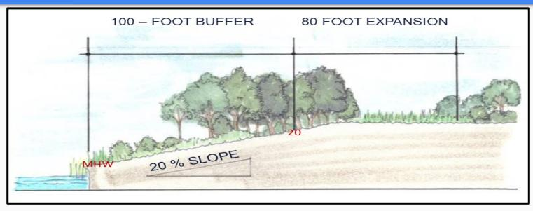
Expansion for steep slopes of 15% or greater: 4 feet for every 1% of steep slope. In this example, the 100-foot Buffer is contiguous to 20% slopes; therefore, the Buffer must be expanded an additional 80 feet (4 x 20).
