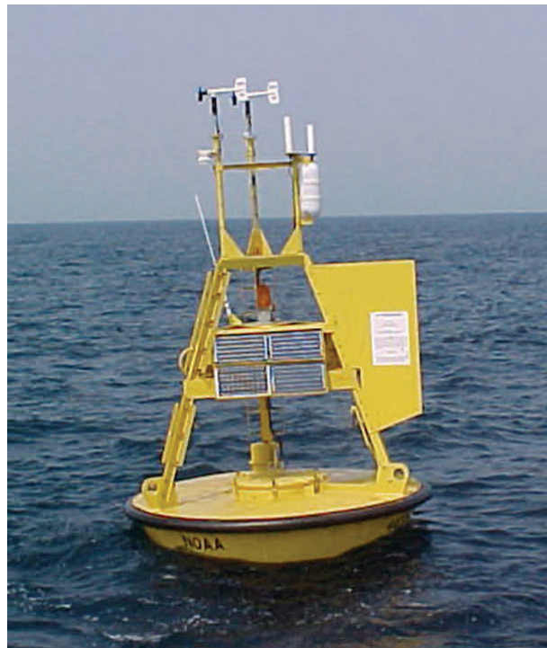
Since 2002, thanks to the NOAA Coastal Storms Program, this data buoy has been gathering information on ocean winds and wave heights to aid mariners and enable forecasters to provide advanced warnings of weather hazards.
