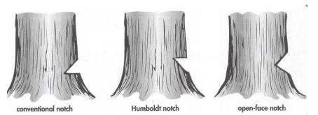
is a directional felling cut facing the direction of fall and consisting of a horizontal face cut and an angled cut below it. A Humboldt cut Copyright International Society of Arboriculture. Used with permission
