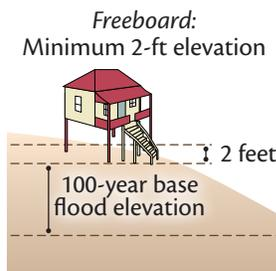
Freeboard is an elevation above a designated high water level. As sea level rises, so will the height of flood levels. The Maryland Climate Action Plan recommends that the lowest horizontal part of a structure within a tidally influenced floodplain be built to allow for two or more feet of freeboard above the 100-year base flood elevation.
