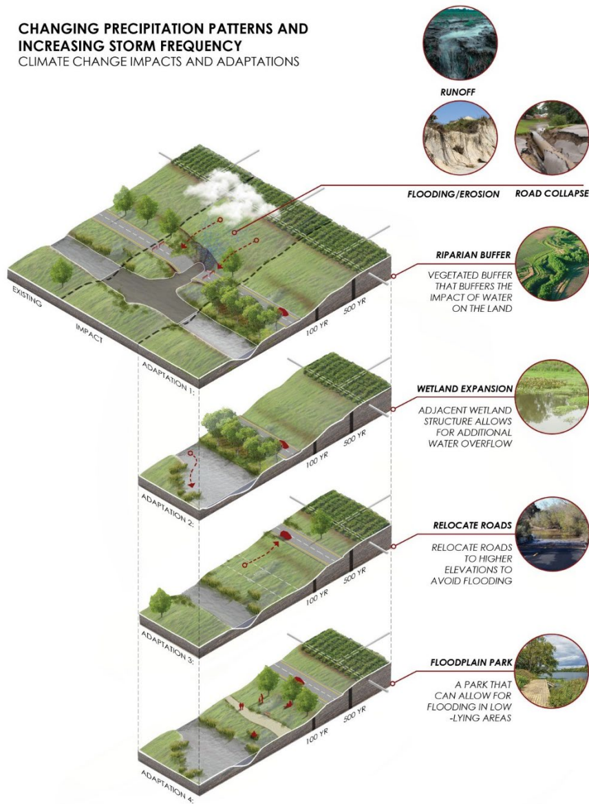
Figure 9: This shows adaptation options for increased flooding of roadways.
