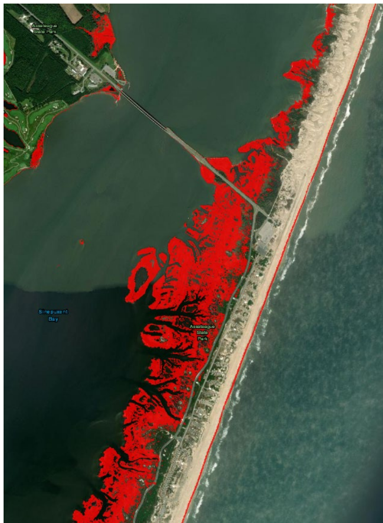
Figure 4: This map shows areas that are currently subject to tidal flooding (in red), often called “recurrent or nuisance flooding.”
