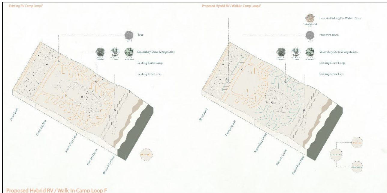
Figure 17: Proposed modifications to campsites to allow for dune migration, decreased sand deposition, and increased usability, UMD.
