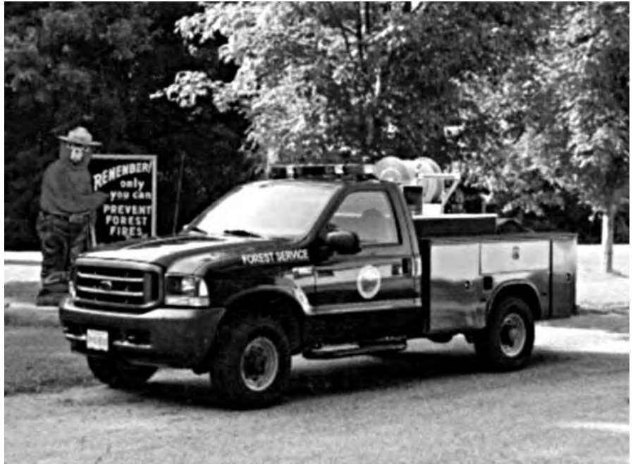
Fig. 28. Forest Ranger Patrol Truck with "utility body" now provides ample storage for today's advanced fire fighting equipment.
