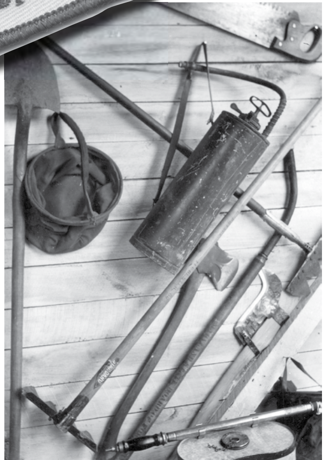
Fig. 21. Early forest fire tools: pointed long-handled shovel, collapsible canvas bucket, hand-pump sprayer, pole axe, backfire torch, brush hook, single handle cross cut saw, 5-gallon back pack water pump, Rich fire rake. Photo by Fred W. Besley, May 1928.
