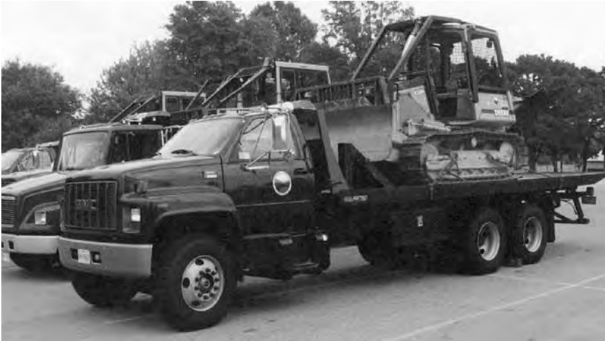
Fig. 48. Today, regionally assigned, radio dispatched, tilt bed trucks quickly transport fire plow tractors with operator protection bars to wildfire locations throughout the State of Maryland.
