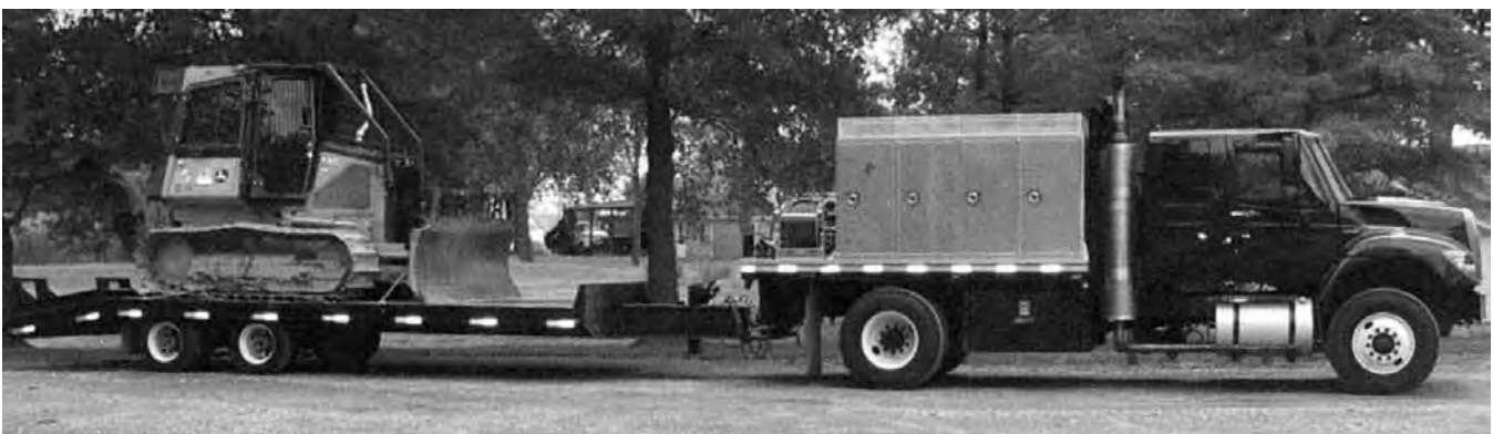
Fig. 49. State-of-the-art wildfire unit "category 4" engine and tanker with the latest Class A foam delivery system for extinguishing wildfires faster and preventing flairups; and also towing a D-14 tractor with fire plow.
