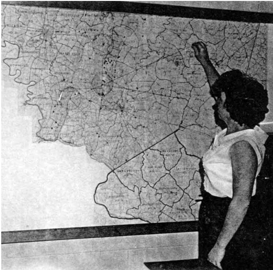
Fig. 18. Carrie Toms, secretary at the Gambrill State Park/High Knob Forest and Park Office, plotting location of a forest fire by pulling the push pins on fishing line along the compass readings reported from three fire towers.
